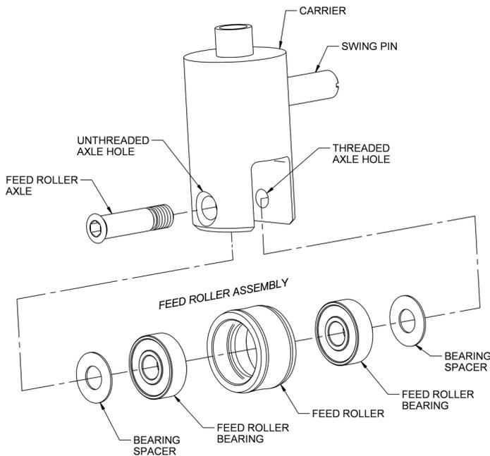
1. Remove the Feed Roller Assembly by unscrewing and removing the Feed Roller Axle.
