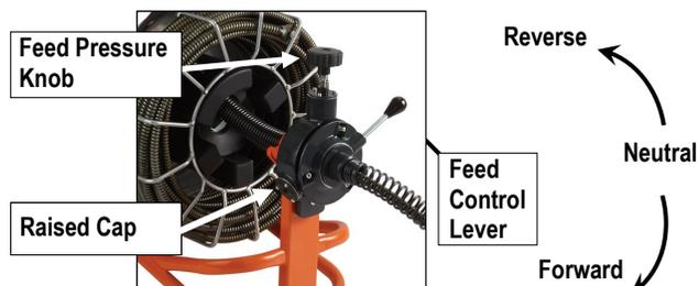
Move lever up to retract cable into drum. When the lever is in the middle (neutral) position, cable will spin in place.
