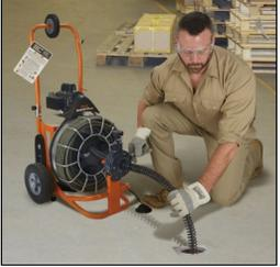
2. Position the air foot pedal for easy accessibility. The machine is designed for one-person operation. Be sure you can quickly remove your foot from the pedal in an emergency.
