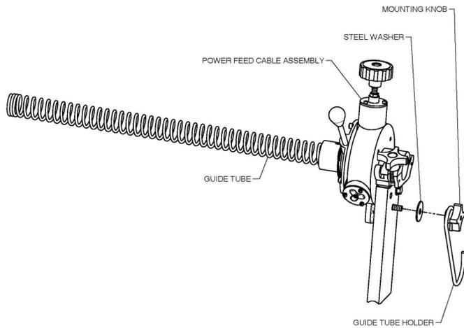
2. To secure the end of the Guide Tube, place it between the frame support tubes.
