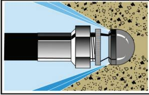
**SPECIALTY NOZZLES:** Spring leader nozzles and down head nozzles are special nozzles to help hose travel through the pipe when there are a lot of Tee's, curves, and bends.
