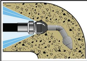
**ROTARY NOZZLES:** Rotary nozzles are useful as a finishing tool. After the line has been cleared, you may switch to the rotary nozzle to more thoroughly clean the walls of the pipe. Use these nozzles only in a predominantly straight run since they are longer than regular nozzles and may get caught in tight bends.
