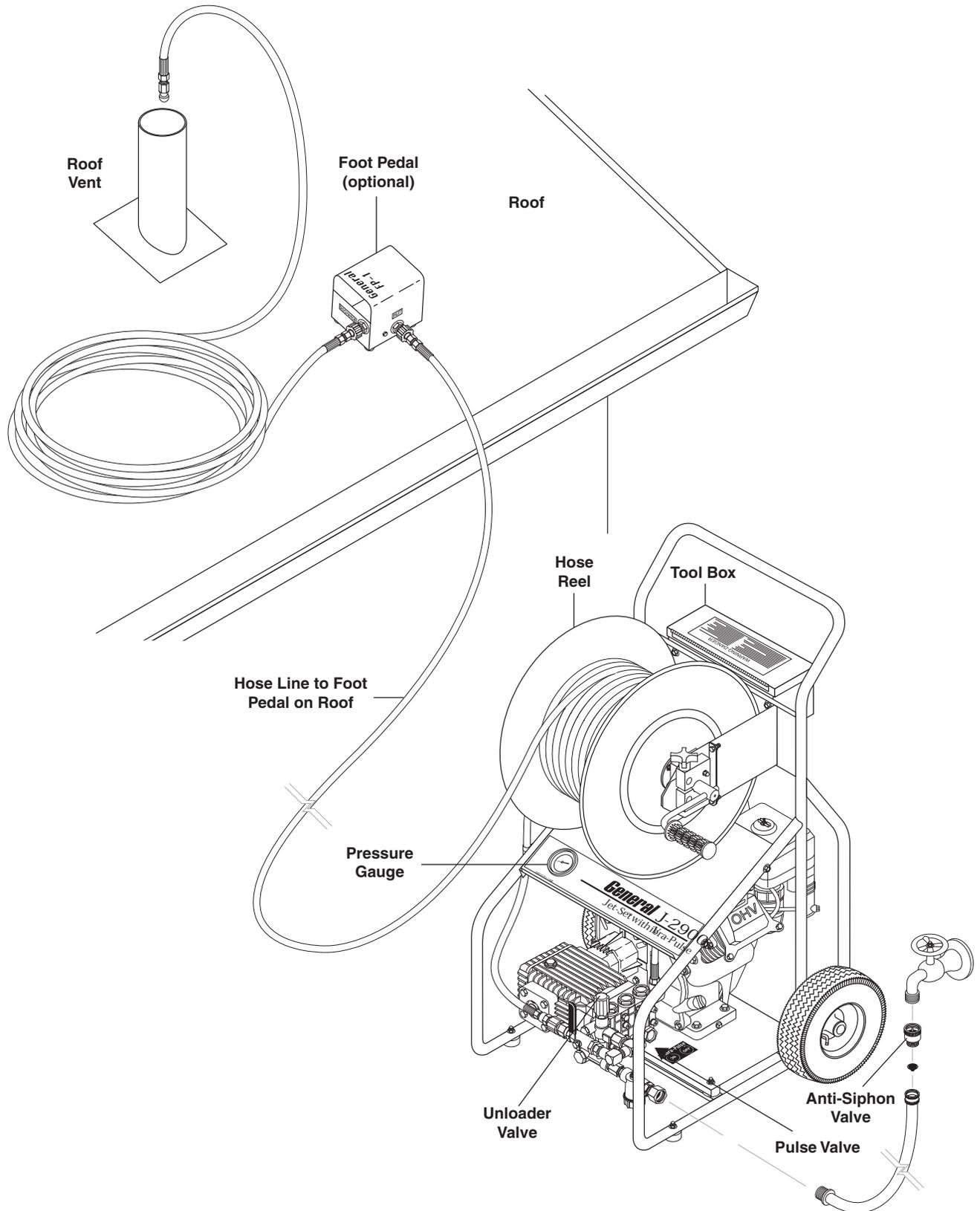
a 3/8" (9.925mm) hose will only lose 25 lbs. (1.7 bar) of pressure over the same length and at the same flow rate. At 4 GPM, a 3/8" hose will lose 90 lbs. (6.2 bar) of pressure over a 100 ft. (30.5m) length. The gauge reflects pressure from the pump only, not pressure at the end of the hose. It is important to select the largest possible hose size in order to have as much pressure as possible at the end of the hose.
