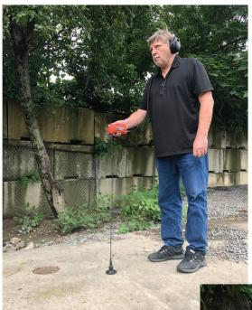
Now, a smaller investment gets you a better method for tracking down water leaks. The new Gen-Ear LE is a simplified, more economical tool with stronger sound amplification than other systems. Use it to pinpoint water leaks in residential and commercial water lines, whether they are under concrete slabs, in walls, swimming pools or hot tubs.
