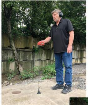
Now, a smaller investment gets you a better method for tracking down water leaks. The new Gen-Ear LE is a simplified, more economical tool with stronger sound amplification than other systems. Use it to pinpoint water leaks in residential and commercial water lines, whether they are under concrete slabs, in walls, swimming pools or hot tubs.
