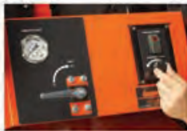
Easily accessible Variable Speed rewind control, along with pressure gauge and output valve mounted between the hose reels.
