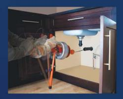
Uni-Stand securely supports your hand-held drain cleaner. Just rock your machine back and forth as you feed the cable into the line.
