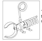
To disconnect, push the coupling key into the hole just below the slot in the female connector, then slide connectors apart
