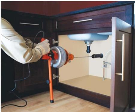
2. Slide the cable into the drain as far as it will go.
