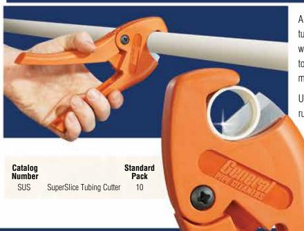
A patented V-point blade pierces hard or soft plastic tubing, then slices through to give a clean, easy cut with virtually no tube deformation. The blade is offset to give you powerful, penetrating action with a minimum of force.
