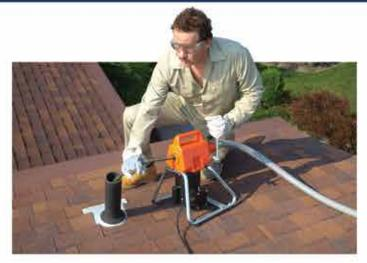
The Root 66 has a wide four point base for greater stability. Its interlocking tubular construction also gives it excellent durability. To protect the gears from dirt and for easier cleaning, the machine has two internal plastic shields. A Ground Fault Circuit Interrupter is standard equipment.
