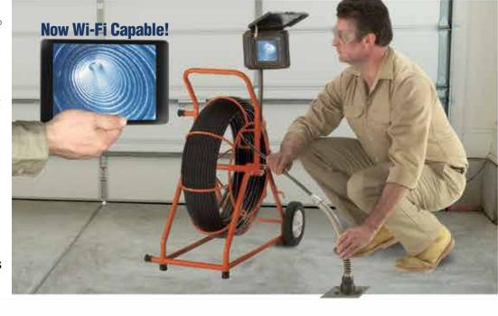
There's lots more, like the LED Dimmer Control, both AC and DC power cords, 2", 3" and 6" Trap Skids, and a 512 Hz transmitter. A video out connection lets you record on an external device.
