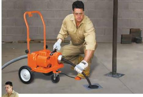
build-ups. For additional protection, the Rodrunner has an adjustable slip clutch, factory set at 18 - 20 ft. lbs.
