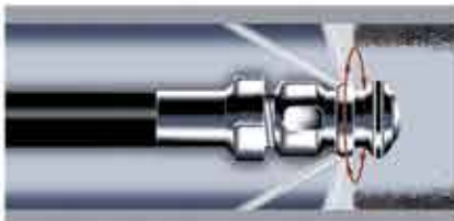
Rotary nozzles scour wall of pipe crystal clear.
