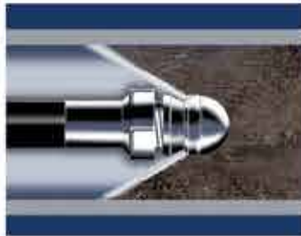
Wide spray flushing nozzle cleans inside of pipe thoroughly,
