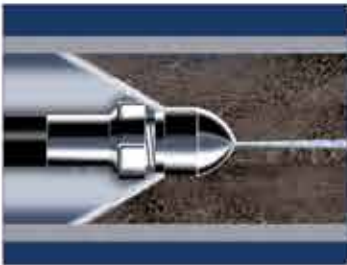
Powerful penetrating nozzle cuts through grease and ice.
