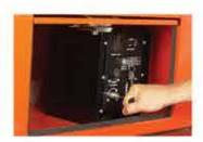
Remote control panel protected inside locked toolbox.
