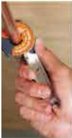
It's quicker than conventional cutters. Just snap it on the tube, close the gate and turn. The cutter wheel automatically tightens as you turn the AutoCut – no knobs to twist. The cutter wheel is spring loaded to provide a constant cutting pressure, so you'll never accidentally crimp the tubing.
