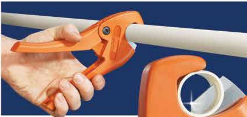
A patented V-point blade pierces hard or soft plastic tubing, then slices through to give a clean, easy cut with virtually no tube deformation. The blade is offset to give you powerful, penetrating action with a minimum of force.
