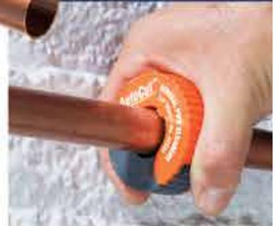
The AutoCut has long lasting hardened steel cutting wheels that are easy to replace when the time comes. Keep a 1/2", 3/4" and 1" AutoCut in your tool box. Watch out though, they'll spoil you.
