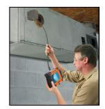
NOTE: The micro push rod is designed to be used in 1-1/2" to 3" lines ONLY. Do not use it in larger or smaller lines, or you may damage the push rod.
