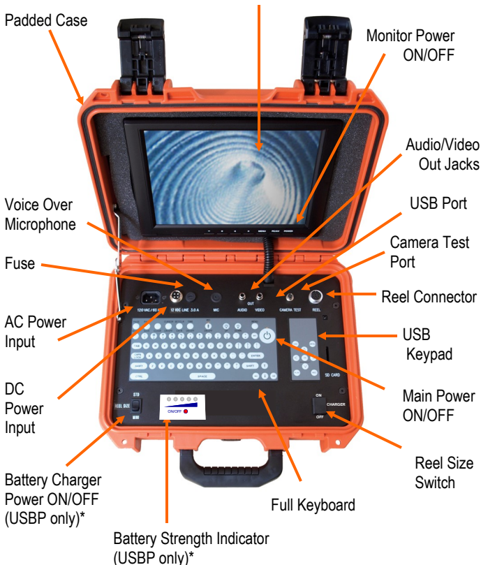
10.4" LCD Color Monitor (sun-readable on USBP)
