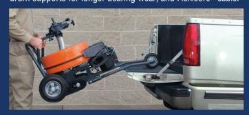
One person easily loads the Speedrooter XL onto a truck. The swept-back handles and loading wheel give you the needed leverage.
