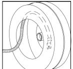
Note: The cable should lay in the drum in a clockwise direction.
