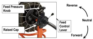
Move lever up to retract cable into drum. When the lever is in the middle (neutral) position, cable will spin in place.
