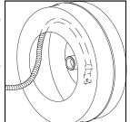
**NOTE:** The cable must lay in the drum in the correct direction or it will tangle in the drum.
