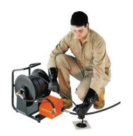
For remote operation, pull the hose from the hose reel to the drain site. Attach the hose to the inlet of the pedal. The pedal is designed for 3/8" hose fittings. If using a 1/4" hose, use the AD-1 adapter, as well. Then, attach the smaller hose (1/8" or 1/4") to the outlet side of the pedal. Use the smaller hose to clear the drain line.
