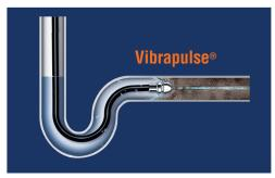
This is what separates General's Jet-Set from ordinary pressurewashers. Vibra-pulse breaks the initial tension between the surface of the hose and the walls of the pipe, helping the hose slide around tight bends and propel it farther down the line. Vibra-pulse increases the cleaning power of electric jets, and is particularly useful in jetting around bends in small drains.
