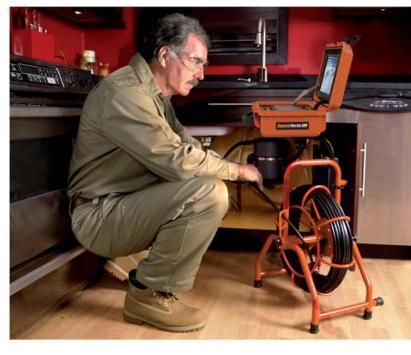
The fully adjustable docking arm lets you mount the monitor on a big capacity reel loaded with Gel-Rod® push-rod and a color selfleveling camera. With this easily maneuverable, all-in-one package you're all set to trouble-shoot 3" to 10" lines with the standard reel. or inspect 2" to 4" lines with the mini-reel.
