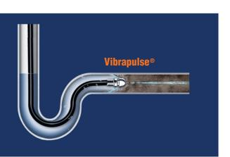
This is what separates General's Jet-Set from ordinary pressurewashers. Vibra-pulse breaks the initial tension between the surface of the hose and the walls of the pipe, helping the hose slide around tight bends and propel it farther down the line. Vibra-pulse increases the cleaning power of electric jets, and is particularly useful in jetting around bends in small drains.
