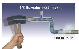
The Ram has a self-contained pump and pressure gauge, so you can hit the stoppage with just the right amount of force. You get instant impact with no build-up of pressure in the plumbing system. The force is transmitted through water, so it's not affected by stacks or vents.
