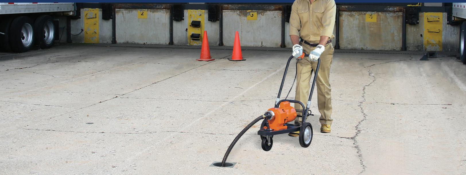
This machine is almost as easy to run as a lawn mower. You push eight or ten foot cable sections into the line until you reach some resistance. Then attach the rear cable coupling to the machine, stand behind it, and turn it on. Watch the cable feed itself into the line. When a section has run into the drain, attach another one and keep going. This self-feeding feature also works to pull sections out of the line.
