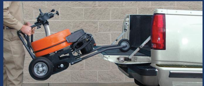
One person easily loads the Speedrooter XL onto a truck. The swept-back handles and loading wheel give you the needed leverage.
