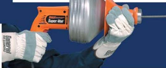
Pull Cable out of drum. Slide Shield **Back** to grip cable.
