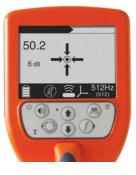
Simply follow the arrows to find the exact spot. When you are over the NULL point, the screen will produce this display.
