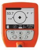
you will have the exact location of the transmitter and the lay of the pipe.
