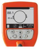
Follow the arrow to pinpoint the location of the transmitter. Simply rotate the flat edge of the locator blade relative to the arrows on the outside of the 'compass' to determine the orientation of the transmitter. When the display shows this graphic:
