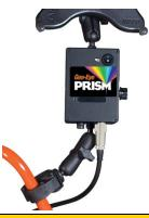
THE AC CORD SHOULD ALWAYS BE PLUGGED INTO THE COMMAND MODULE FIRST, THEN INTO THE WALL.
