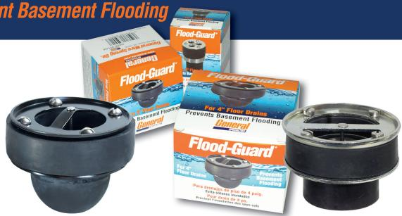
Flood-Guard operates like a check valve to seal off water back-up caused by overloaded sewers. Water flows normally through the drain until the sewer begins to back up. Then the Flood-Guard float rises to seal off the drain opening until the water recedes.
