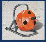
For inside lines up to 3" in diameter. Drum holds 50 ft. x 3/8" Flexicore wire rope center cable. Jacobs hand-tight chuck tightens firmly against the drain snake. Drum can easily be removed for added portability. Includes pneumatic foot pedal for safety and speed control.
