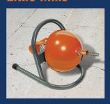
Compact tool offers drain cleaning at a very reasonable price. Drum holds 50 ft. of 5/16" Flexicore wire rope center cable to clear inside lines up to 2" in diameter. Thumbscrew grips cable. Includes pneumatic foot pedal for safety and speed control.
