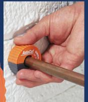
Do stub-out work closer to the wall than conventional pipe cutters because there's no turning handle to get in your way.
