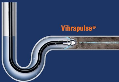
This is what separates General's Jet-Set from ordinary pressurewashers. Vibra-pulse breaks the initial tension between the surface of the hose and the walls of the pipe, helping the hose slide around tight bends and propel it farther down the line. Vibra-pulse increases the cleaning power of electric jets, and is particularly useful in jetting around bends in small drains.
